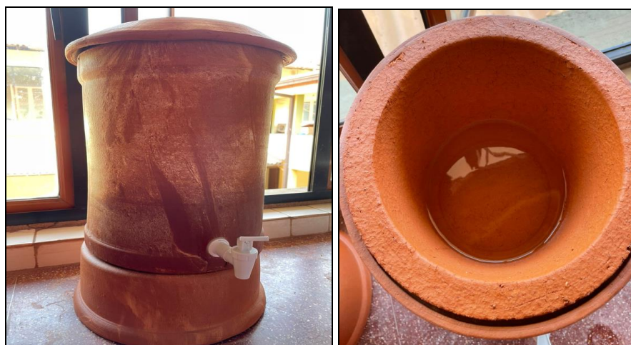
Fig. 5 Laterite soil-based household water purification cylinder (Outside view and inside view)
